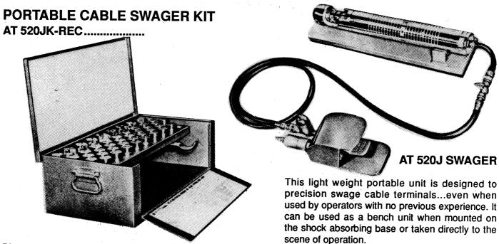
Dies are for standard MS Sleeve Type and Ball End Terminals. Cut-off and trim dies are manufactured in sizes to cut cable up to 1/4" in diameter without fraying or crushing wire strands. The kit is furnished with swager and all dies (1/16-3/16).
