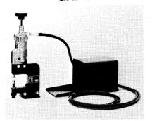
3000CS and 6000CS are excellent bench tools for light to medium assembly work. The foot control frees the assemblers hands to position the workpiece. With the unique stroke control capability, the operator can easily make minute adjustments and always be assured of smooth, even pressure.
