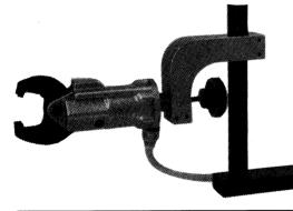
The Model 3000 AS and 6000 AS alligator type featuring unique adjustable stroke control. It is designed for simple bench mounting. It is portable and easy to set up, making it ideally suited to work in confined areas. It is perfect for riveting and inserting captive hardware. Shipped with bench mount, foot control and guard plus all hoses and connectors ready to operate. See optional alligator jaw table on page 1.
