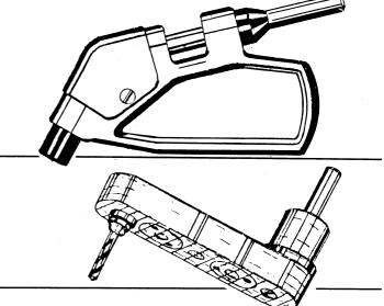
**TERRY NO. T 25 -** Flat Offset Drilling Attachment (Short Handle) with 1/4"-28 threaded spindle. The 2-5/16" offset gives greater access to tight places. Needle Bearings in the Handle, Hardened Alloy Steel Drive Shaft and Gears make this a most durable tool.
